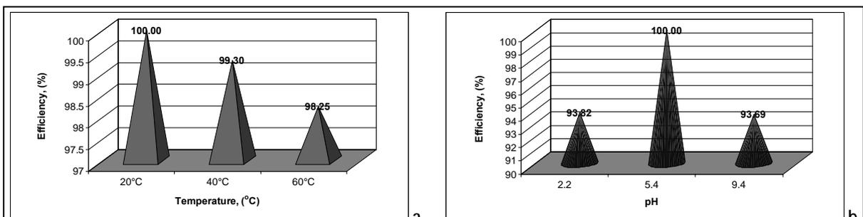
**Fig. 2.** Influence of the temperature (a) and pH (b) over the cadmium maximum removal efficiency on immobilized bentonite sample (10 g),  $C_i = 48 \text{ mg Cd}^{2+}/\text{L}$ ,  $\text{pH} = 5.4$  (fig. a),  $T = 20^\circ\text{C}$  (fig. b).
