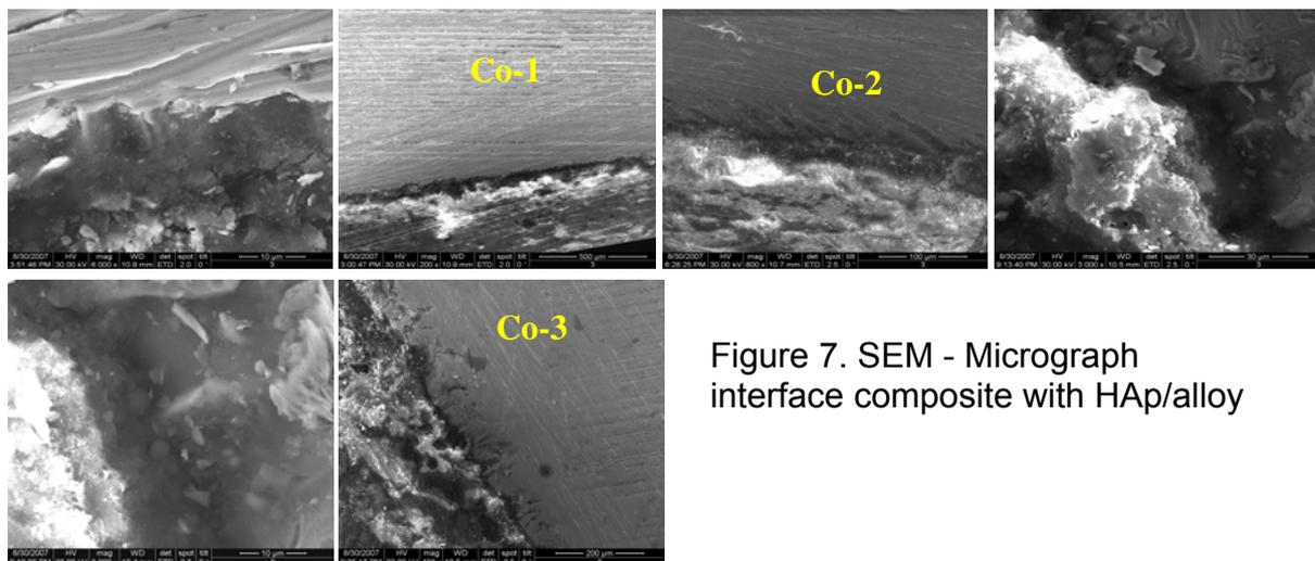
Figure 7. SEM - Micrograph interface composite with HAp/alloy
