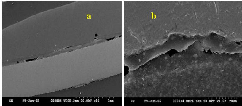
Figure 8. SEM - Micrograph interface composite C20/alloy
