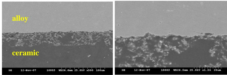
Figure 5. SEM Co-2 alloy/ceramic interference
