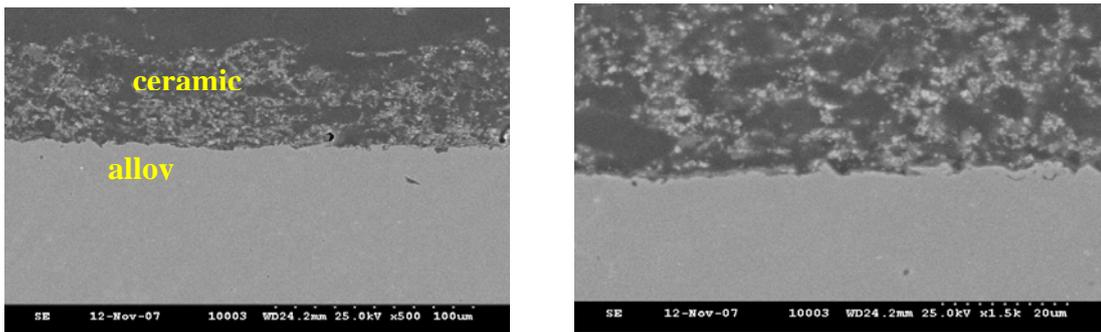
Figure 4. SEM Co-1 alloy/ceramic interference
