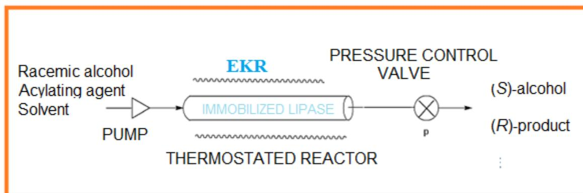
Figure 1. Testing the enzymatic processes in continuous flow reactors
