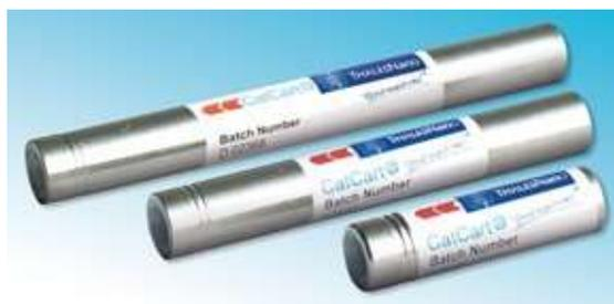
As reactors SynBioCart (30 mm×3 mm ID PTFE) columns were used, which were filled with the immobilized catalyst (120 mg CaLB-SWCN<sub>COOH</sub> or 110 mg of immobilized racemization agent) in fixed bed, using as sealing system teflon and metallic sieves seals which permit the uniform distribution of the flow.
