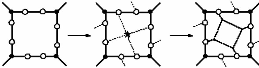
**Figure 10.** The Capra operation on a square face.
