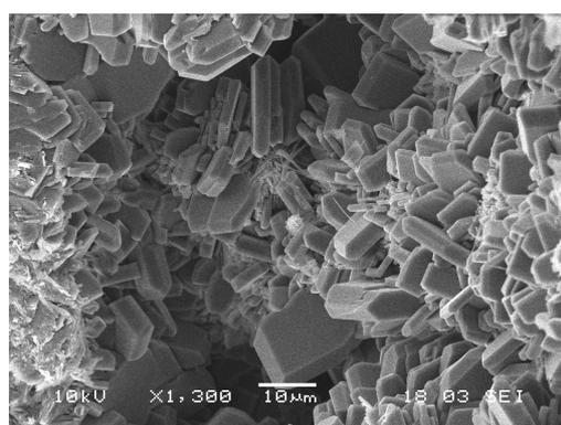
**Figure 4.** SEM image of a tuff sample from Aluniș (Cluj County). Clinoptilolite euhedral tabular crystals.
