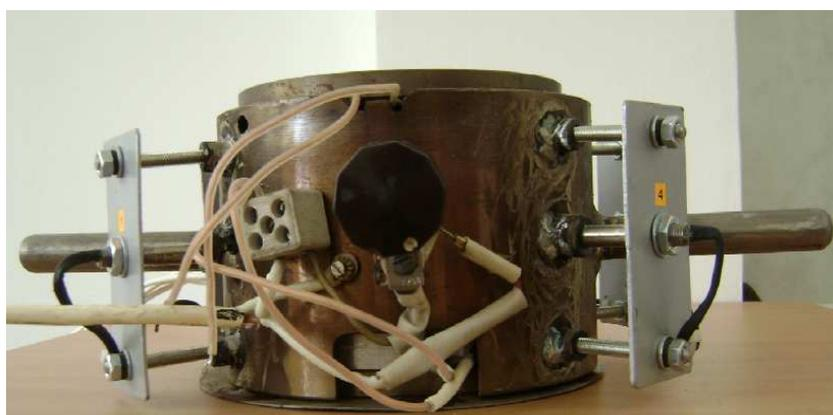
**Figure 1.** The plates fabrication mould.
