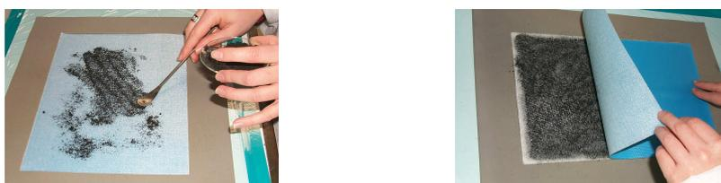
**Figure 4.** Manual doping of impregnated laminates.
