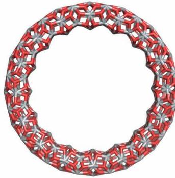
**Figure 1.**  $\text{TiO}_2$  nanotube (a) and nanotorus (b).
