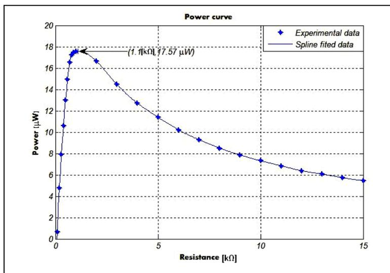
**Figure 4.** Power curve 0.05M sodium acetate solution
