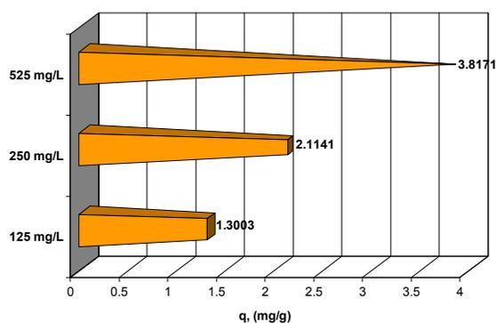
**Figure 5.** Influence of the initial zinc concentration over the adsorption capacity, in zinc removal process on 2 grams of Orașul Nou bentonite sample in dynamic regime (3D shaker).
