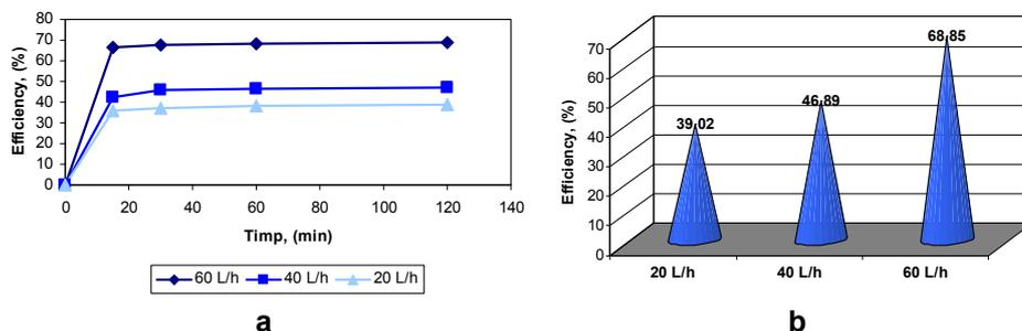
**Figure 4.** Variation (a) and maximum values (b) of overall efficiency in the phenol CWAO process, at different air flows and constant temperature, 80°C, for  $\text{Fe}^{(3+)}$ -DCA catalyst (0.1 g catalyst and  $C_i = 1000 \text{ mg phenol/dm}^3$ ).
