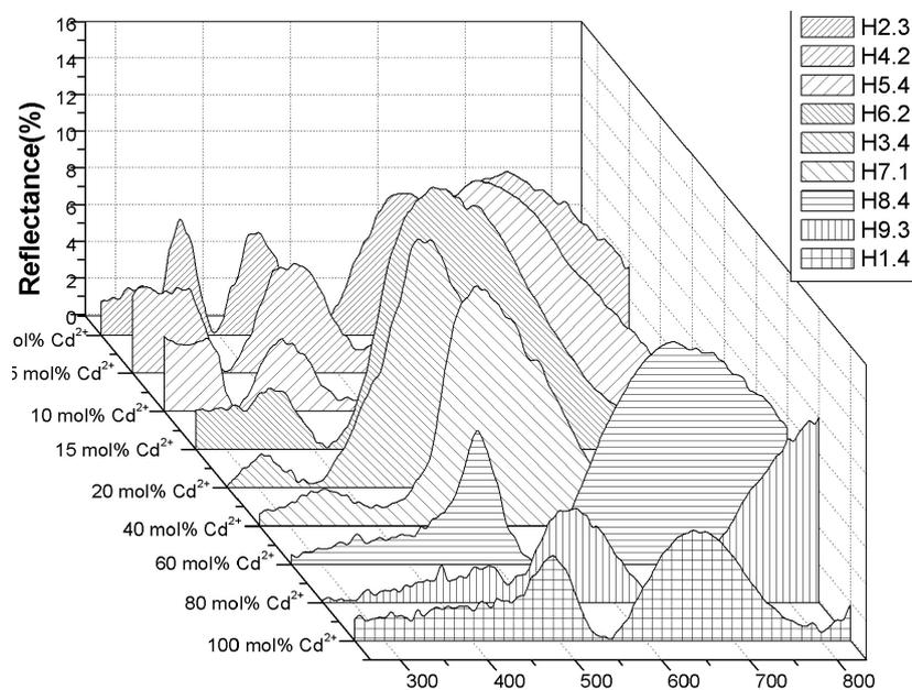
**Figure 4.** Specular reflectance spectra of ZnCdS thin films obtained from chemical bath with different Cd<sup>2+</sup> amounts
