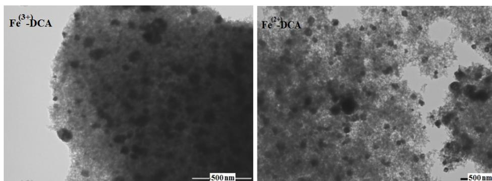
Figure 1. TEM images of iron doped carbon aerogels.
