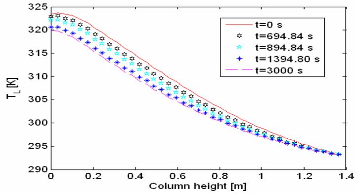
Figure 6. Variation of liquid's temperature ( $F_L = F_L + 20\%$ )
