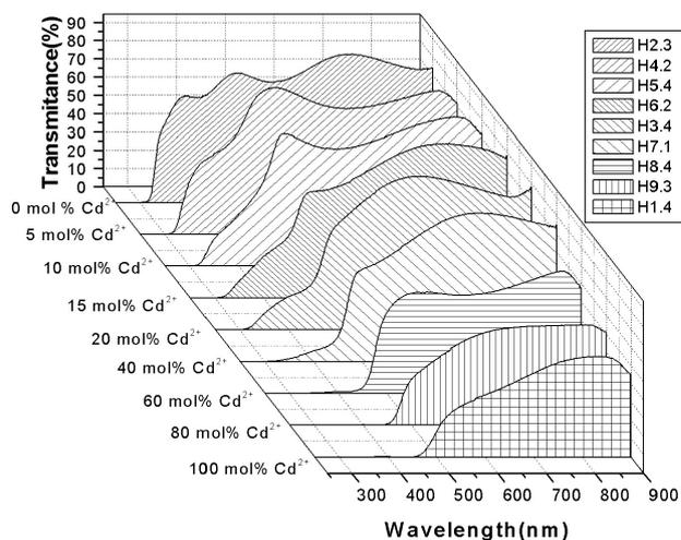
**Figure 2.** Transmittance spectra of ZnCdS thin films obtained from chemical bath with different  $\text{Cd}^{2+}$  amounts
