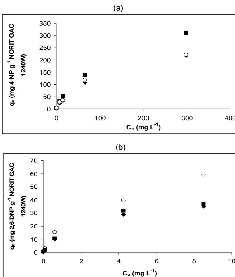
**Figure 1.** The fit of experimental data ( $\blacklozenge$ ) to Langmuir ( $\blacksquare$ ) and Freundlich ( $\circ$ ) models at  $25^\circ\text{C}$  for: (a) 4-nitrophenol and (b) 2, 6-dinitrophenol in water.
