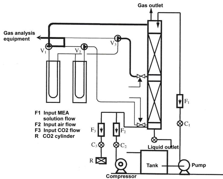
**Figure 1.** Gas – liquid packed absorption column
