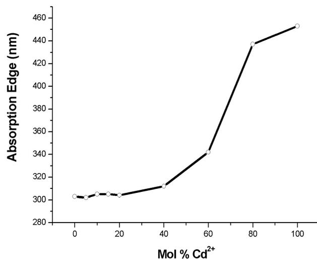
**Figure 3.** Variation of absorption edge position of ZnCdS thin films with  $\text{Cd}^{2+}$ -amount from chemical bath
