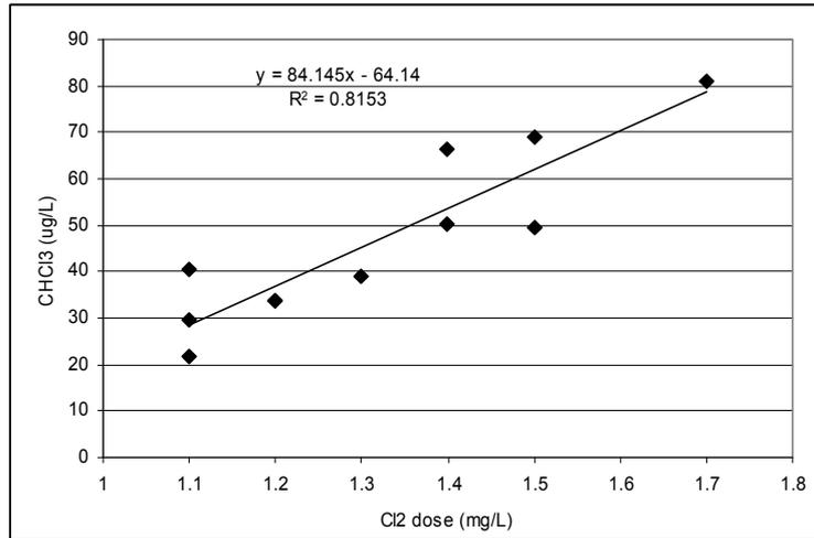
**Figure 1.** Chlorine dose as function of CHCl<sub>3</sub> concentration in Gilau WTP
