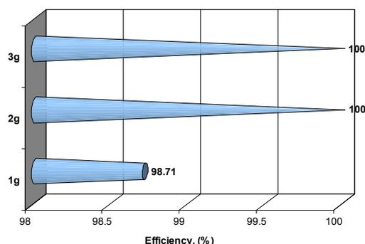
**Figure 7.** Influence of the bentonite quantity over the maximum removal efficiency, in zinc removal process on Oraşul Nou bentonite sample in dynamic regime (3D shaker),  $C_i = 125 \text{ mg Zn}^{2+}/\text{g}$ .
