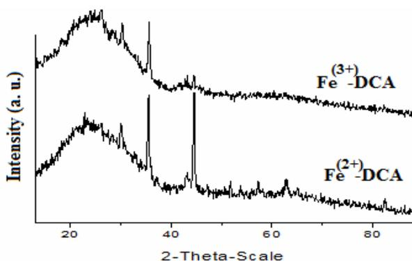
Figure 2. XRD patterns of iron doped carbon aerogels.
