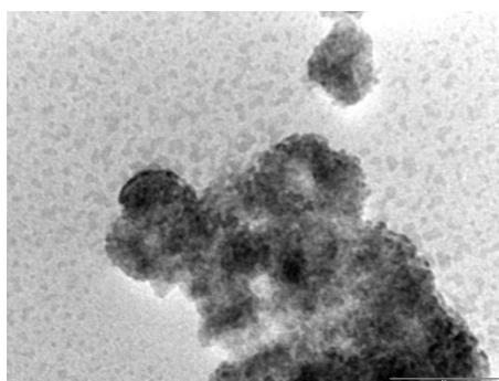
**Figure 6.** TEM image of ZnS:Mn<sup>2+</sup> (scale bar=50 nm)
