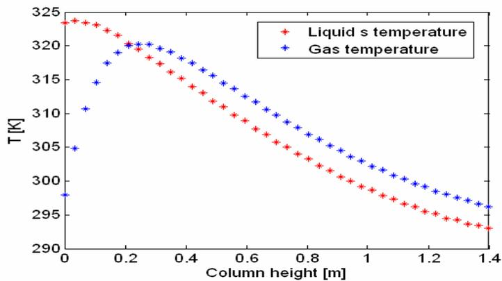
**Figure 5.** Temperature profile along the column height
