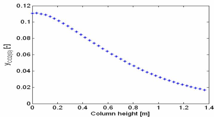
Figure 2. CO<sub>2</sub> concentration (in gas phase) along the column height
