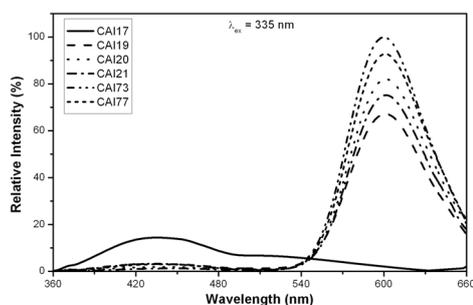
**Figure 3.** Emission spectra of  $ZnS:Mn^{2+}$  powders obtained from acetate mixtures with various  $Mn^{2+}$  concentration.
