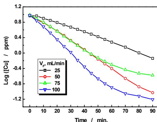
**Figure 2.** The evolution in time of the copper concentration for different volume flow rate (ε<sub>W.E.</sub> = -200 mV/RE; 7.5 mM Na<sub>2</sub>SO<sub>4</sub>)
