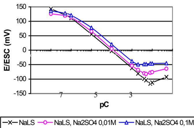
**Figure 1.** The influence of the ionic strength on the response functions of the laurylsulphate sensible electrode:
