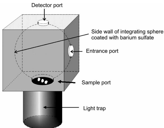
**Figure 1.** The schematic drawing of the integrating sphere
