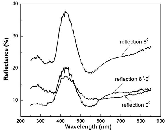
**Figure 4.** Reflectance spectra for the multilayer  $\text{WO}_3$  film (R415) measured on ITO face.
