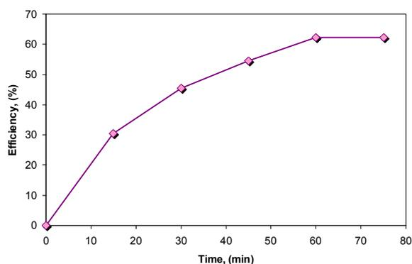
**Figure 10.** Removal efficiency evolution in time during cadmium removal process on Orașul Nou bentonite sample in dynamic regime (3D shaker),  $C_i = 25$  mg Cd<sup>2+</sup>/L, 2 g bentonite, 20 ml solution.
