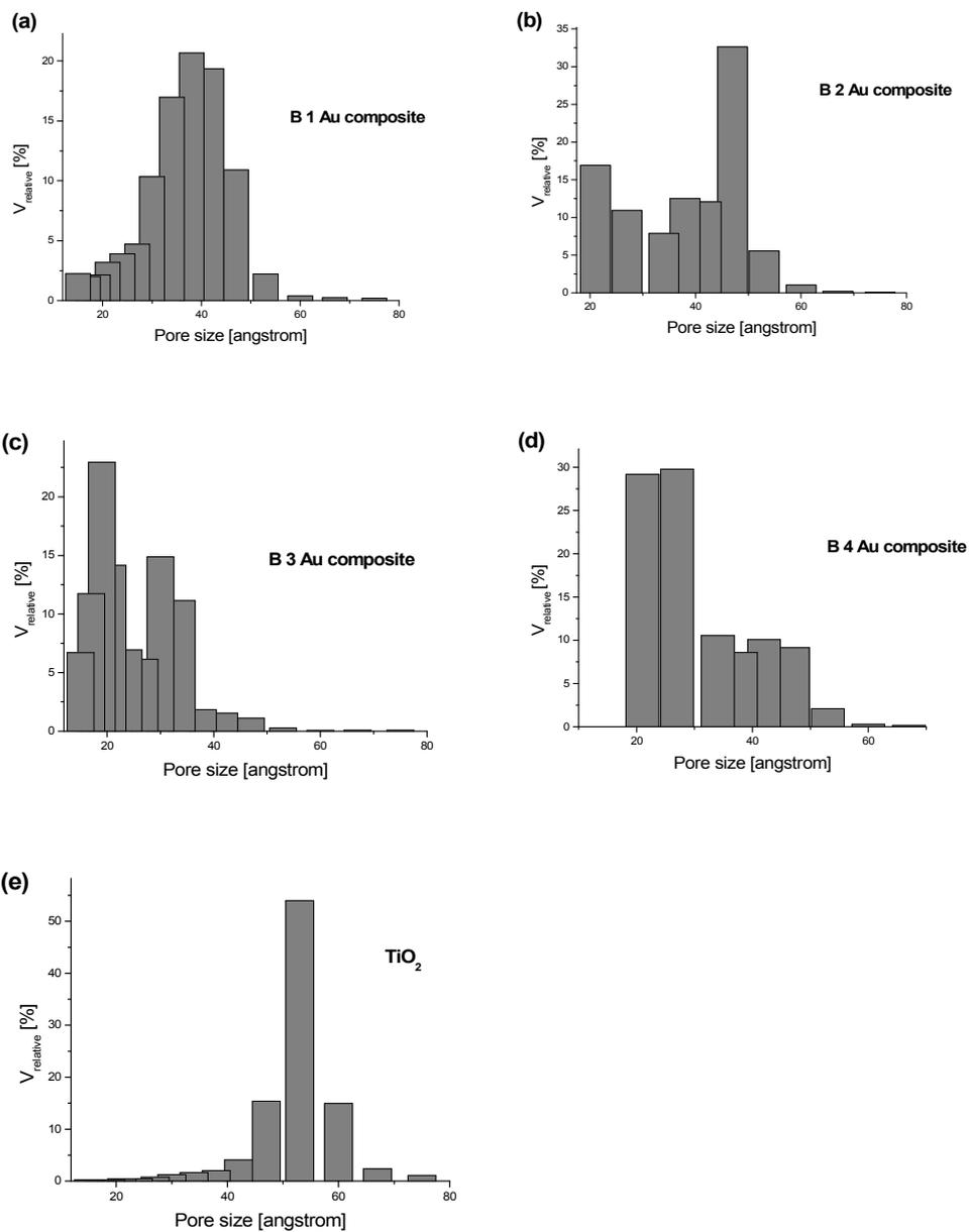
**Figure 2A.** Influence of the Au loading on the composites pore structure.
