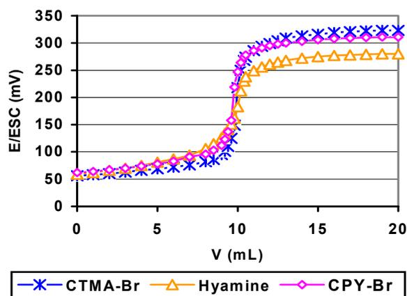
**Figure 3.** Influence of the titrating agent on the potentiometric titration curve (titration of 50 mL NaLS  $10^{-3}$  M with different cationic surfactants,  $5 \times 10^{-3}$  M) Indicating electrode: TCMA-LS membrane plasticized with DOS
