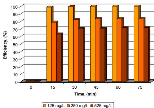
**Figure 4.** Influence of the initial zinc concentration over the removal efficiency evolution in time, during zinc removal process on 2 grams of Orașul Nou bentonite sample in dynamic regime (3D shaker).
