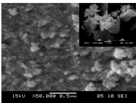
**Figure 5.** SEM image of ZnS:Mn<sup>2+</sup> sample (inset scale bar = 1  $\mu\text{m}$ )
