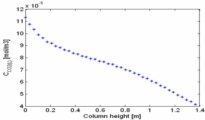
**Figure 4.** CO<sub>2</sub> concentration (in liquid phase) profile along the column height
