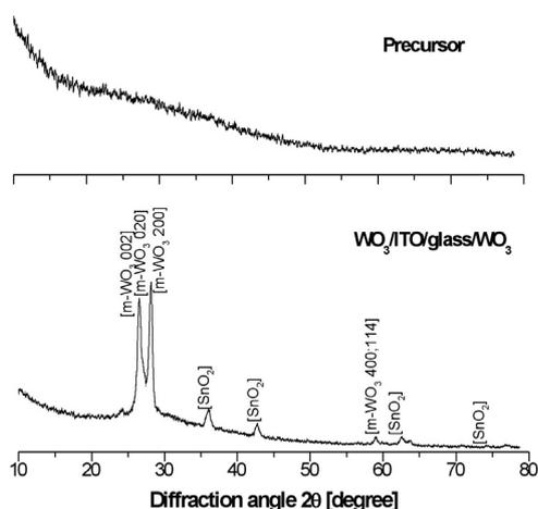
**Figure 6.** XRD patterns for PTA precursor and the corresponding heterostructure WO<sub>3</sub>/ITO/Glass/WO<sub>3</sub> (film R415).
