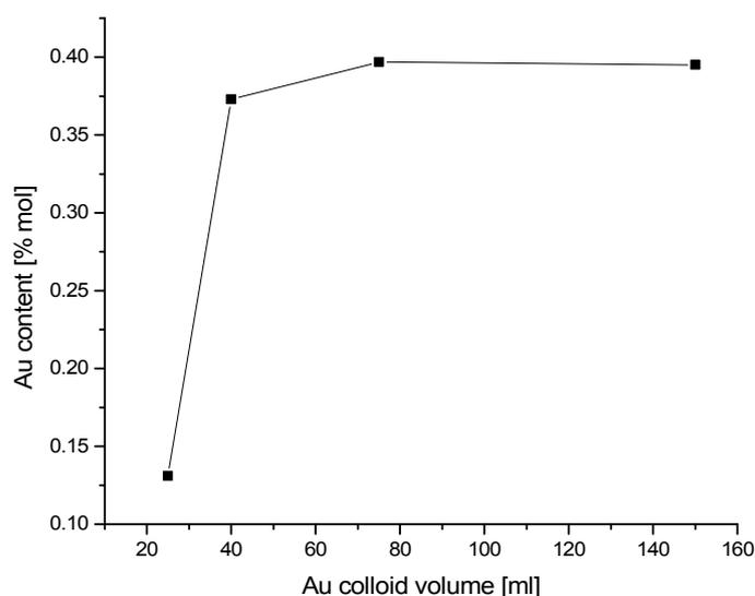
**Figure 1.** Dependence of Au content on the Au colloid volume used in TiO<sub>2</sub> gel impregnation
