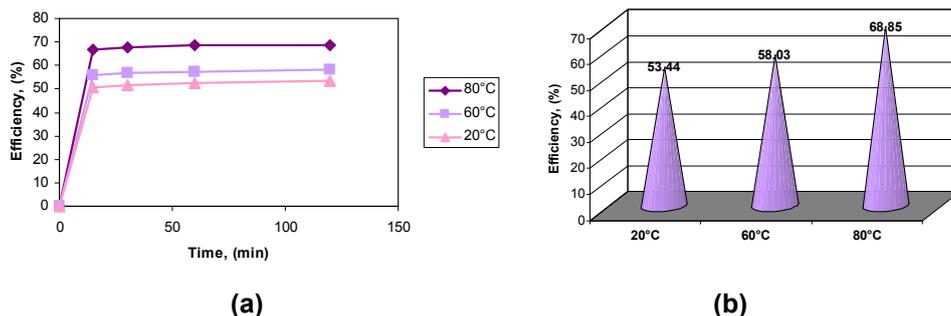
**Figure 3.** Variation (a) and maximum values (b) of overall efficiency in the phenol CWAO process, at different temperatures and constant air flow, 60 L/h, for  $\text{Fe}^{(3+)}$ -DCA catalyst (0.1 g catalyst and  $C_i = 1000 \text{ mg phenol/dm}^3$ ).
