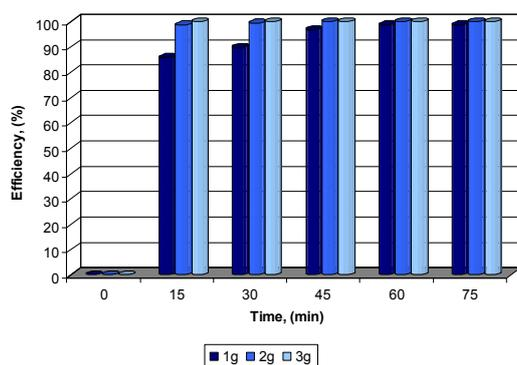
**Figure 6.** Influence of the bentonite quantity over the removal efficiency evolution in time, during zinc removal process on Orașul Nou bentonite sample in dynamic regime (3D shaker),  $C_i = 125 \text{ mg Zn}^{2+}/\text{g}$ .
