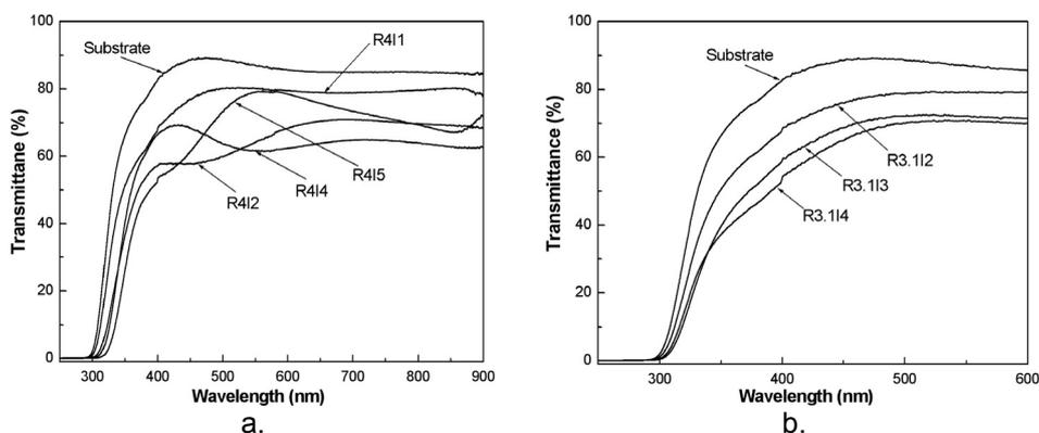
**Figure 3.** Transmission spectra of WO<sub>3</sub> films obtained in different conditions: a) multilayer films treated at 350°C; b) monolayer films annealed at 250 – 550°C.
