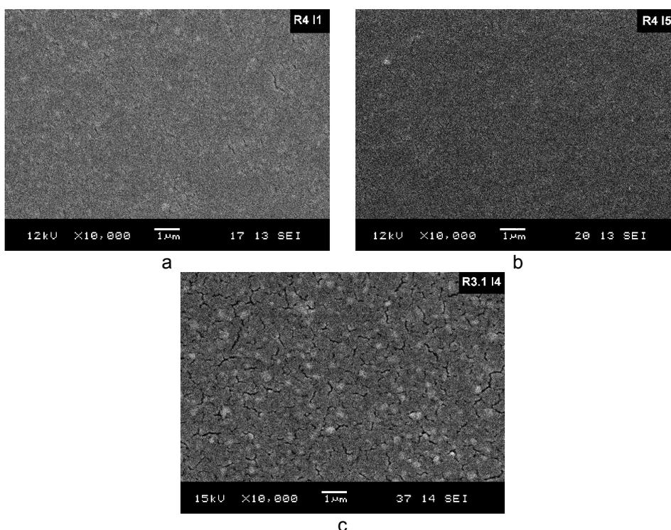
**Figure 7.** SEM images of WO<sub>3</sub> film surface: (a) one layer (350°C) (b) five layers (350°C) and (c) one layer (550°C).
