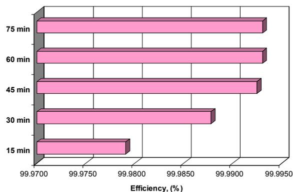
**Figure 9.** Removal efficiency evolution in time during lead removal process on Orașul Nou bentonite sample in dynamic regime (3D shaker),  $C_i = 54$  mg Pb<sup>2+</sup>/L, 2 g bentonite, 20 ml solution.
