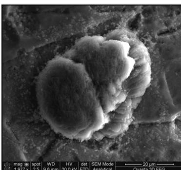
**Figure 5b.** Manganese dioxide germination on Ti–after S2 step; Electrolyte: 1M H<sub>2</sub>SO<sub>4</sub> + 6g/L Mn<sup>2+</sup>, pH≈~0.5, sweep rate 2mVs<sup>-1</sup>
