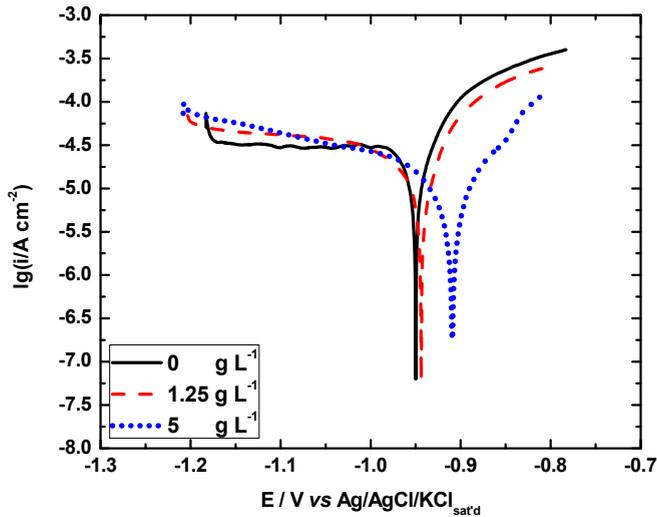
**Figure 5.** Polarization curves ( $\pm 200$  mV vs OCP) for Zn and Zn-CeO<sub>2</sub>-ZrO<sub>2</sub> deposits with various concentrations of nanoparticles
