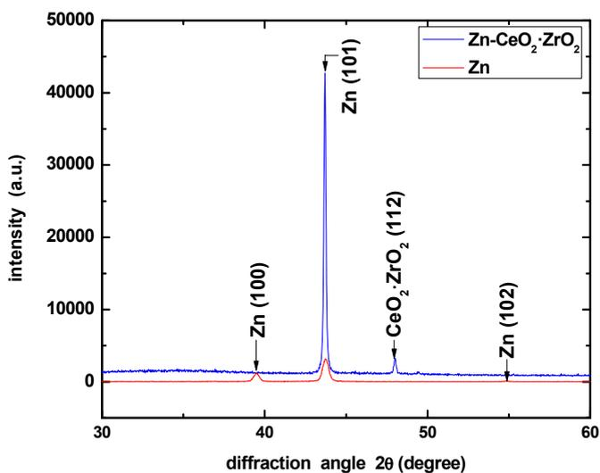
**Figure 3.** X-ray Diffraction results for the Zn and Zn–CeO<sub>2</sub>·ZrO<sub>2</sub> deposits, 1.25 g L<sup>-1</sup>
