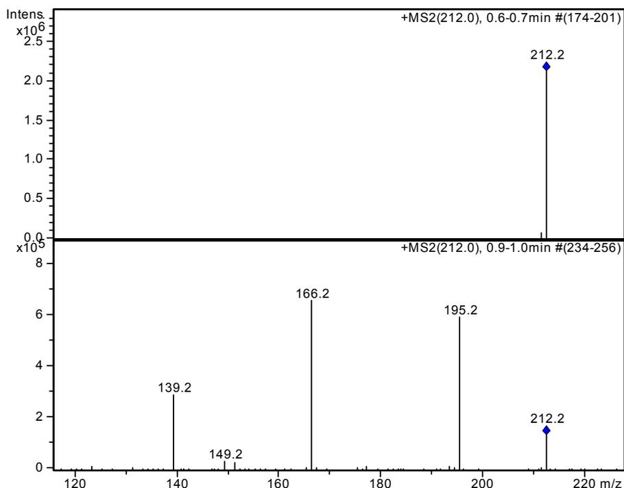
**Figure 3.** Mass spectra of methyldopa obtained by electrospray ionisation in positive ion mode at the collision energy of 1.2 V: (up) full-scan spectrum with molecular ion  $[M+H]^+$  ( $m/z$  212.2); (down) MS/MS reactive spectrum (after fragmentation into monitored ions:  $m/z$  195.2, 166.2, 139.2).
