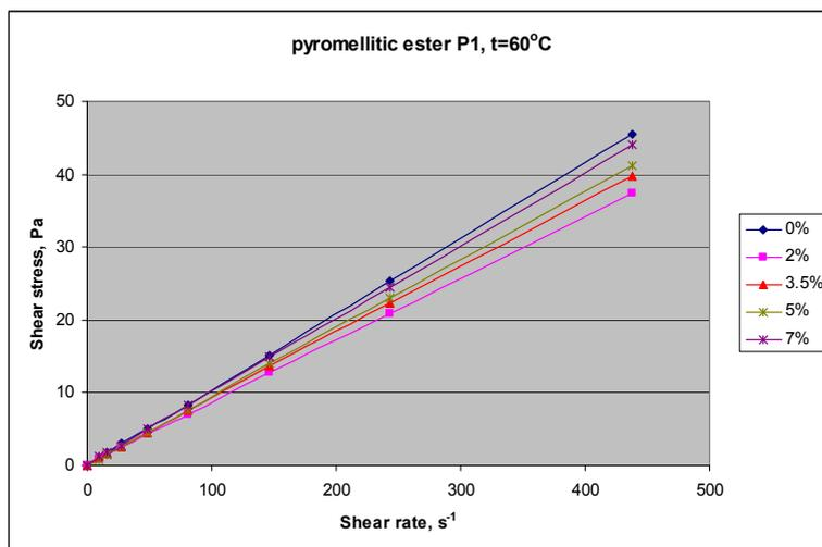
**Figure 2.** Dependence  $\tau = f(\dot{\gamma})$  for samples A0-A4
