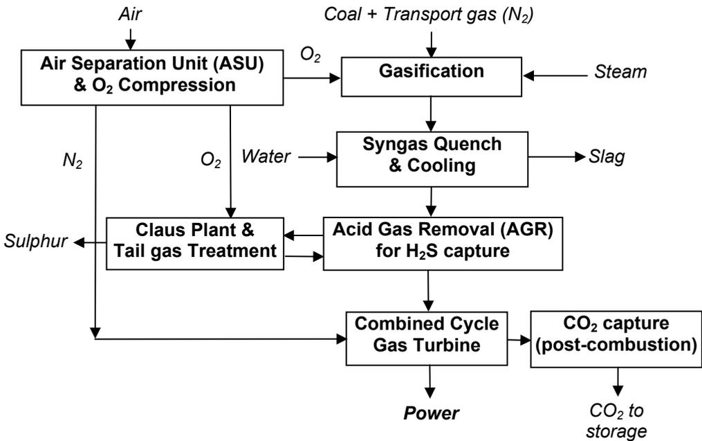
**Figure 2.** Layout of IGCC scheme for power production with CO<sub>2</sub> post-combustion capture
