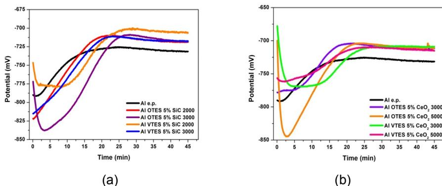
**Figure 3.** Variation of potential in time for Al e.p., Al can and Al with silanes modified with SiC (a) and with CeO<sub>2</sub> (b) in H<sub>3</sub>PO<sub>4</sub> 3M
