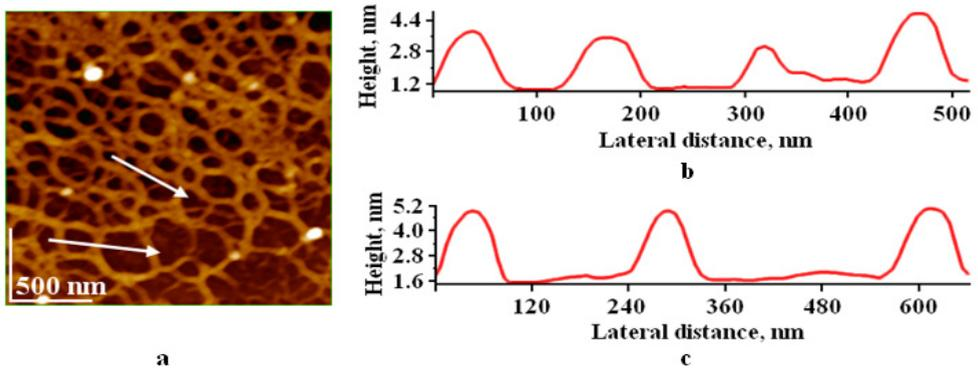
**Figure 4.** Collagen-APTES self-assembled patterns, for volume ratio of 1:2, used in spreading solution, at the air/water interface. AFM images on LB layer transferred on glass, at 25 mN/m: 2D-topography (a); two cross section profiles (b and c), along the 2 arrows given in image (a). Scanned area  $2\mu\text{m} \times 2\mu\text{m}$ . RMS 1.5 nm. Average pore diameters (b and c), from about 30 nm, 160 nm to 210 nm. COLL fiber thickness is almost constant of about  $70 \pm 8$  nm.
