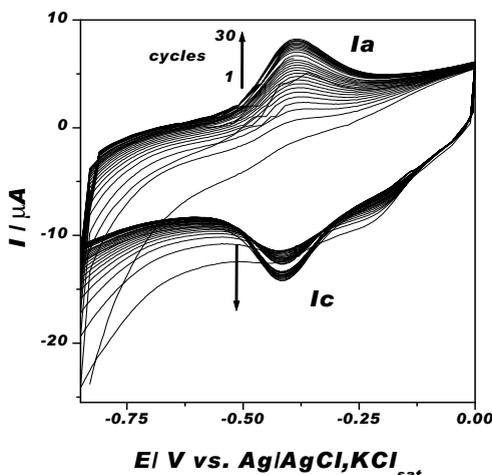
**Figure 1.** Preparation of G/polyHm modified electrode by cyclic voltammetry. Experimental conditions: 0.5 mM Hm in 0.05 M TRIS buffer + 0.1 M KBr, pH 8; starting potential,  $-0.85 \text{ V}$  vs. Ag/AgCl, KCl<sub>sat</sub>; scan rate,  $0.05 \text{ V s}^{-1}$ ; number of cycles, 30; deaerated solution (with N<sub>2</sub>).
