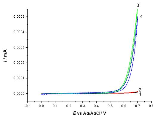
**Fig. 4.** The voltammograms of PIGE modified electrodes in contact with 1 M  $\text{KOH}$  + 1 M  $\text{CH}_3\text{OH}$ . 1-blank electrode; 2- $\text{YFeO}_3$ ; 3- $\text{YCo}_{0.5}\text{Fe}_{0.5}\text{O}_3$  and 4- $\text{YCoO}_3$ .
