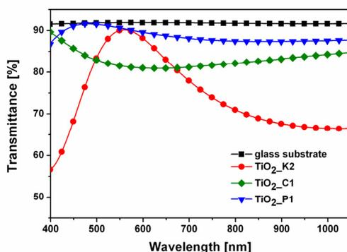
**Figure 1.** Transmittance spectra of the uncoated glass substrate, of the double-layered TiO<sub>2</sub> (TiO<sub>2</sub>\_K2), and monolayered CTAB (TiO<sub>2</sub>\_C1) and Pluronic (TiO<sub>2</sub>\_P1) templated porous TiO<sub>2</sub> coated samples.
