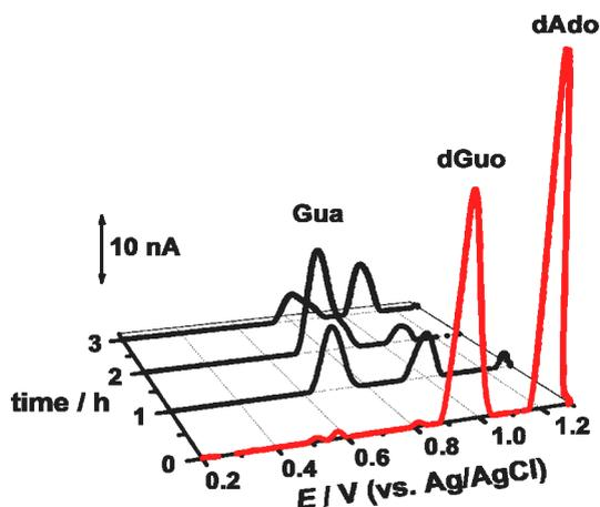
**Figure 8.** 3D plot of baseline subtracted DP voltammograms of multilayer (—) dsDNA-electrochemical biosensor control and (—) after incubation in  $2.5 \text{ mg mL}^{-1}$  RTX in phosphate buffer pH = 7.0 during 0, 1, 2 and 3 h. From reference [23] with permission.
