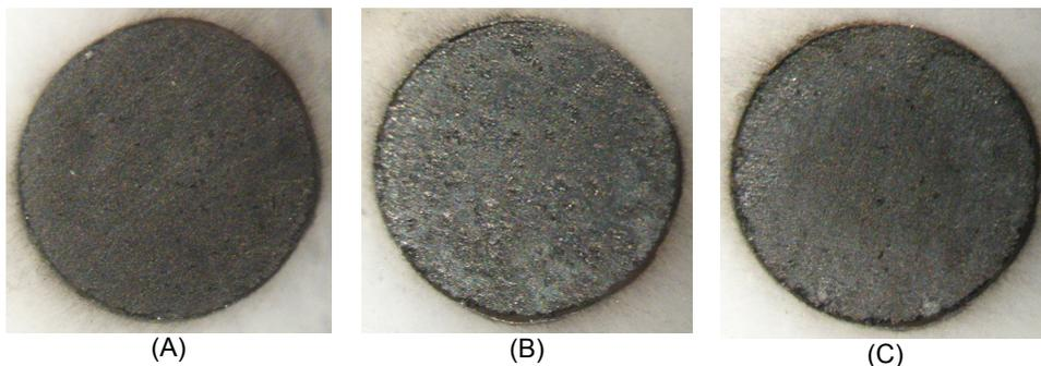
**Figure 5.** Microscopic images of SG/Pb II: the unmodified SG surface (A), after depositing a *approx.*  $2 \mu\text{m}$   $\text{PbO}_2$  layer on the surface (B) and after the completion of the measurements in the  $0.2 \text{ M}$  vanadium in  $2 \text{ M}$   $\text{H}_2\text{SO}_4$  solution (C).
