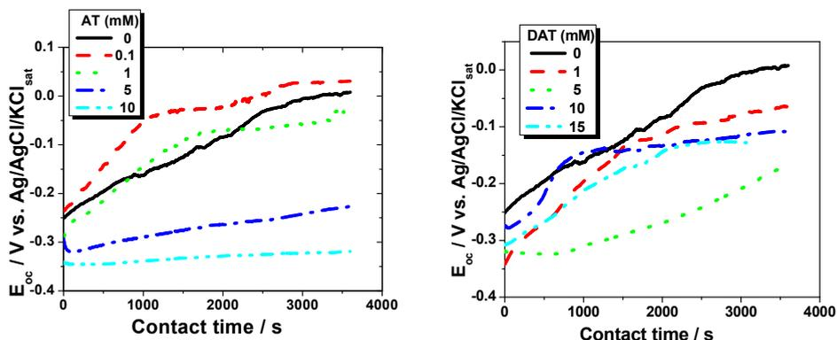
**Figure 1.** Time-variation of the open-circuit potential for bronze during its immersion in the corrosive media (pH 4), in the absence and in the presence of thiadiazole derivatives at various concentrations.
