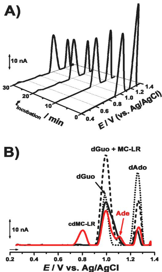
**Figure 5.** DP voltammograms with: **A)** the dsDNA-electrochemical biosensor in buffer pH = 4.5 incubated for different times in 30  $\mu\text{M}$  MC-LR and **B)** GCE in 50  $\mu\text{g mL}^{-1}$  dsDNA solution in pH = 4.5 0.1 M acetate buffer ( $\cdots$ ) before and after incubation with 30  $\mu\text{M}$  MC-LR during ( $\cdots$ ) 0, ( $\text{---}$ ) 6 and ( $\text{---}$ ) 24 h. From reference [15] with permission.
