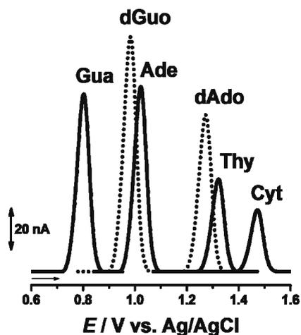
**Figure 1.** DP voltammograms base-line corrected at the GCE in solutions of: 10  $\mu\text{M}$  guanine (Gua), guanosine (dGuo), adenine (Ade), adenosine (dAdo), and 50  $\mu\text{M}$  thymine (Thy) and cytosine (Cyt) in pH = 4.5 0.1 M acetate buffer.
