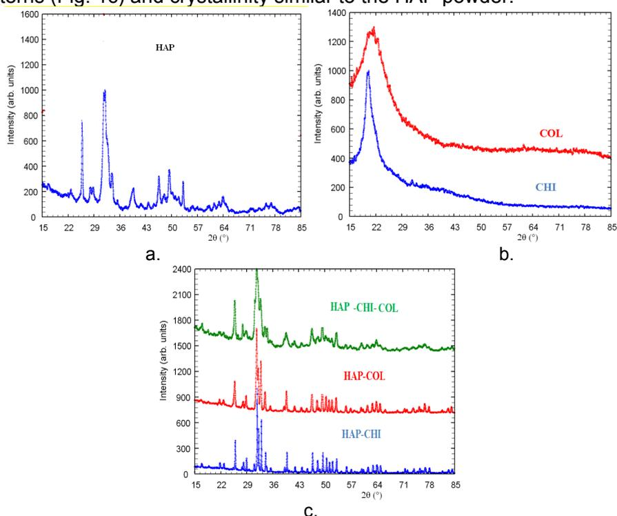
**Figure 1.** X- Ray powder diffraction patterns of HAP (calcined at 650 °C) (a), COL and CHI samples (b), and HAP-CHI (93:7), HAP-COL (70:30) and HAP-CHI-COL (68.5 :5.5 :26) powders (c).
