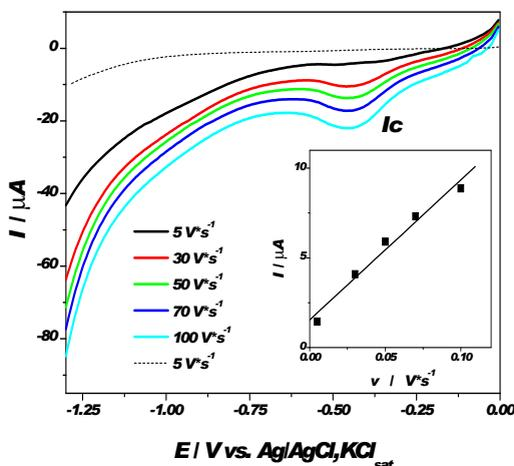
**Figure 2.** Voltammetric response of G (thin dash line) and G/polyHm (thick lines) electrode at different scan rate. Inset:  $I$  vs.  $v$  dependence. Experimental conditions: electrolyte, 0.05 M phosphate buffer + 0.1 M KBr, pH 8; starting potential, 0 V vs.  $\text{Ag/AgCl, KCl}_{sat}$ ; deaerated solution (with  $\text{N}_2$ ).
