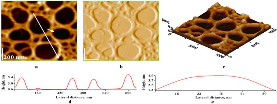
**Figure 3B.** COLL-APTES self-assembled patterns. 2D- topography (a), amplitude (b), 3D topography (c); two cross section profiles (d and e), along the 2 arrows given in image (a); Scanned area  $1\mu\text{m} \times 1\mu\text{m}$ ; RMS 1.9 nm on scanned area (a). Details as in Fig. 3A. Porous layer analysis: average pore diameters (d), from about 40 nm, 150 nm to 240 nm. COLL fiber thickness is almost constant of about  $70 \pm 6$  nm (an example is given in (e) cross section profile).
