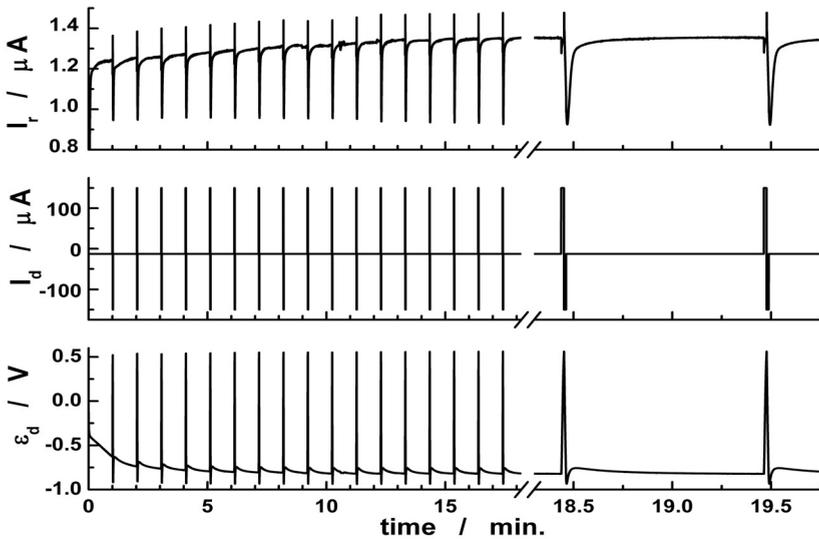
**Figure 2.** The evolution of  $I_r$ ,  $I_d$  and  $\varepsilon_d$  during 20 cycles of galvanostatic auto-adaptive EA and HPE. ( $V_F = 1.42$  mL/min.;  $\varepsilon_{AS, MAX} = +0.5$  V;  $\varepsilon_{PRS, MIN} = -0.8$  V;  $T_{PS} = 60$  s;  $I_{AS} = +150$   $\mu$ A;  $I_{PRS} = -150$   $\mu$ A;  $I_{PS} = -13$   $\mu$ A)
