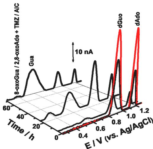
**Figure 6.** DP voltammograms baseline corrected in 0.1 M phosphate buffer pH = 7.0 using a multilayer dsDNA-electrochemical biosensor (—) control and after (—) 10 min, 4, 24 and 72 h in 250  $\mu$ M TMZ solution. From reference [17] with permission.
