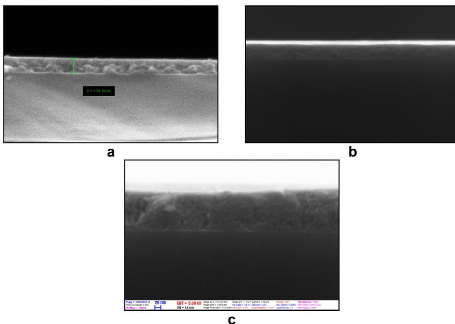
**Figure 2.** The FESEM images of the compact (a), CTAB templated (b) and Pluronic templated (c) TiO<sub>2</sub> layers on silicon substrate.
