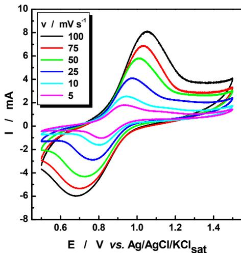
**Figure 1.** CV curves recorded in 0.1 M V<sup>IV</sup> and 0.1 M V<sup>V</sup> in aqueous 2 M H<sub>2</sub>SO<sub>4</sub> on a spectral graphite electrode (SG I) at various scan rates, at T = 298 K
