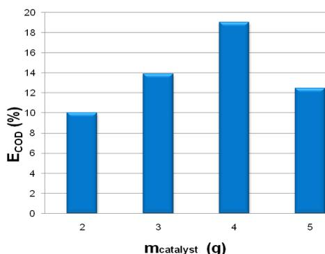
**Figure 3.** Catalyst quantity influence over the COD efficiency variation in the phenol CWAO process, for Cu1-Z catalyst (20 L/h,  $60^{\circ}\text{C}$ , 1000 mg/L, 6 h).
