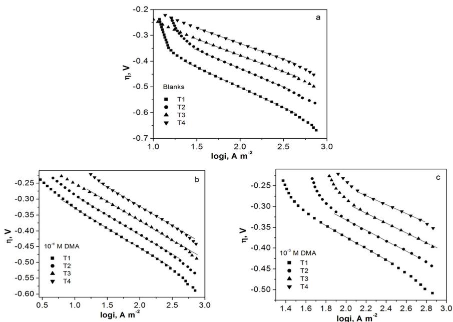
**Figure 2.** Tafel plots for HER on copper electrode in blank 0.5 M  $\text{H}_2\text{SO}_4$  solution (a) and in the presence of different concentrations of DMA:  $10^{-6}$  M (b),  $10^{-3}$  M (c); at different temperatures:  $T_1 = 298$  K;  $T_2 = 308$  K;  $T_3 = 318$  K;  $T_4 = 328$  K.
