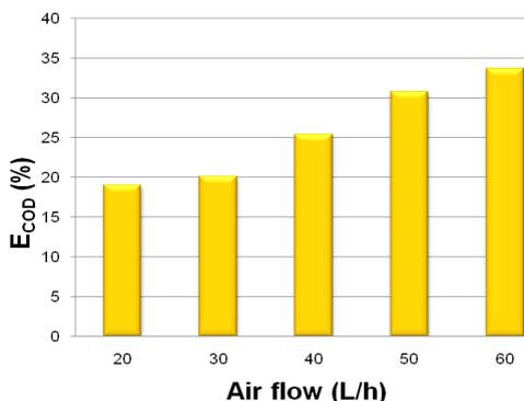
**Figure 2.** Variation of COD efficiency in the phenol CWAO process, at different air flows and constant temperature ( $60^{\circ}\text{C}$ ), for Cu1-Z catalyst (4 g, 1000 mg/L, 6 h).
