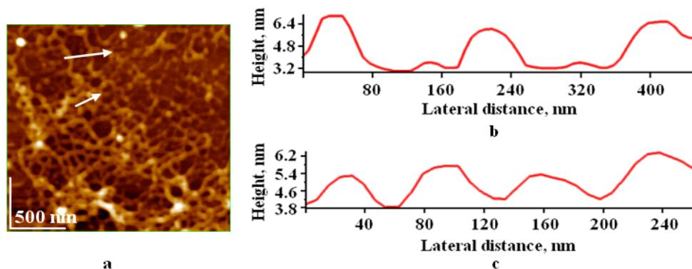
**Figure 5.** Collagen- APTES self-assembled patterns, for volume ratio of 1:3, used in spreading solution. AFM images on LB layer transferred on glass from air/water interface, at 35 mN/m. 2D-topography (a); two cross section profiles (b and c), along the 2 arrows given in image (a); Scanned area  $2 \mu\text{m} \times 2 \mu\text{m}$ ; RMS 1.7 nm. Average pore diameters (b and c), from about 20 nm, 80 nm to 140 nm. COLL fiber thickness is almost constant of about  $70 \pm 10$  nm.
