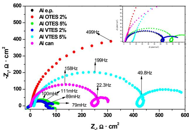
**Figure 4.** Nyquist plots for Al, Al with silane films and commercially available aluminium cans samples in H<sub>3</sub>PO<sub>4</sub> 3M
