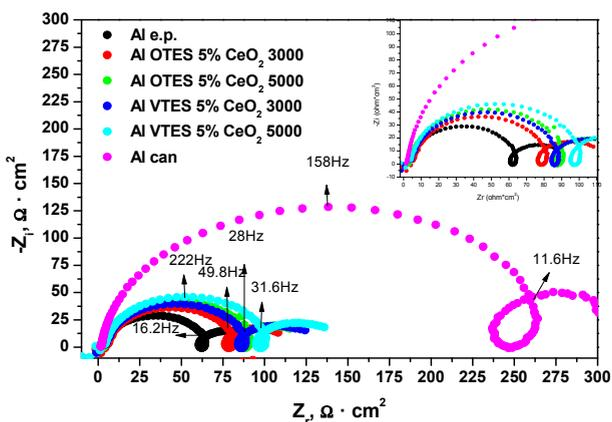
**Figure 6.** Nyquist plots for Al, Al with silane films modified with  $CeO_2$  and commercially available aluminium cans samples in  $H_3PO_4$  3M
