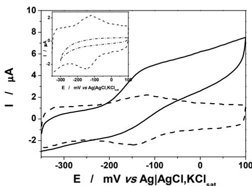
**Figure 3.** Electrocatalytic oxidation of NADH at MB-CA/GCE in the presence of 5 mM NADH and in its absence. Inset: Cyclic voltammogram recorded at MB-CA/GCE (—) and GCE (---). Experimental conditions: scan rate, 20 mV/s; supporting electrolyte, 0.1 M Tris buffer (pH 7); starting potential, -350 mV vs. Ag|AgCl, KCl<sub>sat</sub>.
