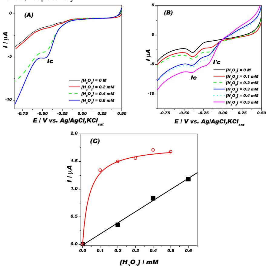
**Figure 3.** Linear scan voltammograms at G (A, ■) and G/polyHm (B, ●) modified electrode for different concentrations of  $\text{H}_2\text{O}_2$  and the corresponding calibration curves for peak  $I_c$  (C). Experimental conditions: electrolyte, 0.05 M phosphate buffer + 0.1 M KBr, pH 8; scan rate,  $0.02 \text{ V s}^{-1}$ ; starting potential, +0.5 V vs. Ag/AgCl,  $\text{KCl}_{\text{sat}}$ ; deaerated solution (with  $\text{N}_2$ ).
