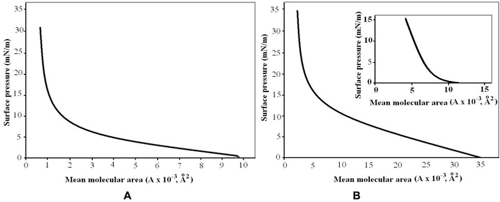
**Figure 1.** Compression isotherms for self-assembled layers: collagen (Fig. 1A), collagen cross-linked by APTES (Fig. 1B, for volume ratio, 1: 1, COLL-APTES) in aqueous solution used for layer spreading, and APTES (inset in Fig. 1B); each layer was spread at the interface between air and aqueous solution of 2M NaCl, at room temperature.
