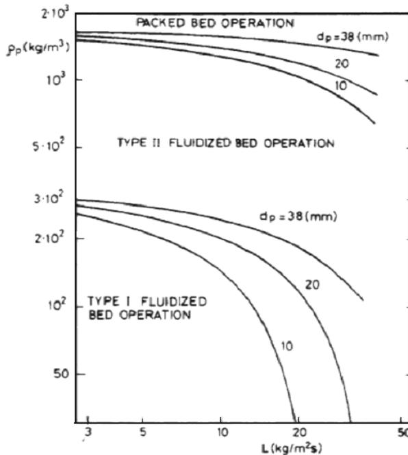
**Figure. 1.** Operating flooding zones in turbulent contact absorber [4].
