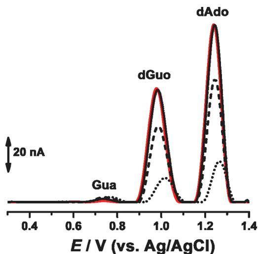
**Figure 7.** DP voltammograms baseline-corrected in pH = 4.5 0.1 M acetate buffer with dsDNA-electrochemical biosensor incubated with 10  $\mu$ M GEM during (—) 0, (---) 15 min, (···) 2 h and (-·-·) 4 h. From reference [20] with permission
