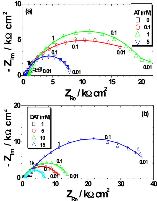
**Figure 3.** Nyquist plots of bronze electrode in the corrosive solution (pH 4), in the absence and in the presence of different concentrations of AT (a) and DAT (b). The symbol (—+—) corresponds to the simulated spectra. Frequencies are expressed in Hz.
