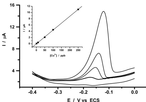
**Figure 1:** Calibration plot for copper (II) in  $0.1$  M  $L^{-1}$  HCl, preconcentration time  $180$  s, initial potential  $-0.6$  V, potential step height  $10$  mV, pulse amplitude  $50$  mV, duration of  $50$  ms, speed of rotation  $300$  rpm. Concentration range  $0.1$  to  $250$  ppb.
