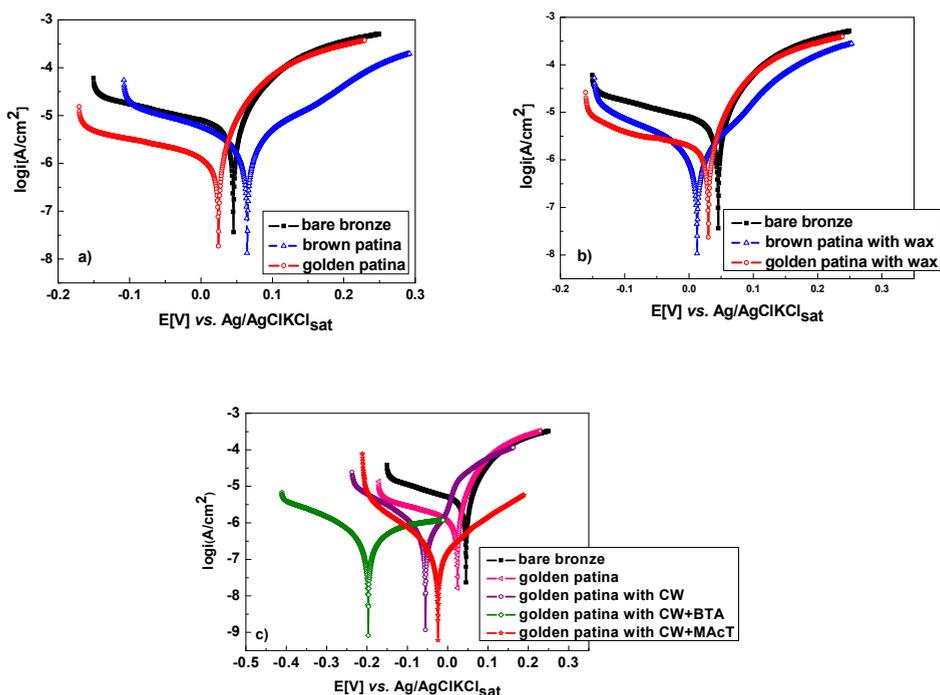
**Figure 1.** The polarization curves ( $\pm 200$  mV vs. OCP) for the bronze covered with: brown and golden artificial patina (a); artificial patina (brown and golden) with WF (b); golden artificial patina with CW in the absence and in the presence of inhibitors (c); Experimental conditions: corrosion solution,  $Na_2SO_4 + NaHCO_3$  (pH 5); potential scan rate, 10 mV / min.
