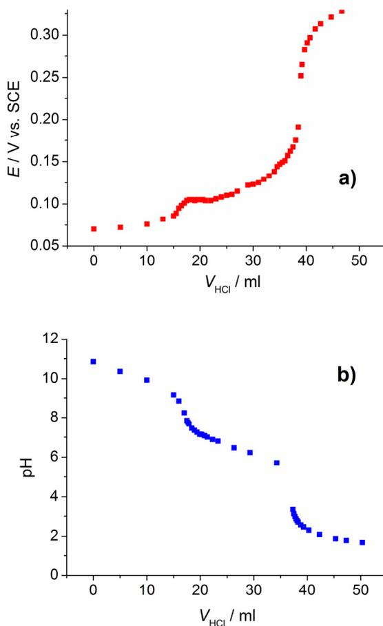
**Figure 2.** Potentiometric titration curves obtained for the titration of 2.5 mmol  $\text{Na}_2\text{CO}_3$  dissolved in  $100 \text{ cm}^3$  water by  $0.1 \text{ mol dm}^{-3}$  HCl at a PIGE (a) and a glass electrode (b), respectively.
