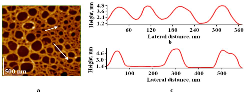
**Figure 3A.** 2D-topography image (a) on LB layer of collagen-APTES self-assembled patterns for volume ratio, 1:1, used as spreading solution (Fig. 1B), transferred on glass from aqueous phase of 2M NaCl, at 15 mN/m. 2D-topography (a); two cross section profiles (b and c), along the 2 arrows given in image (a); Scanned area  $2\ \mu\text{m} \times 2\ \mu\text{m}$ ; RMS 1.7 nm on scanned area (a). Average pore diameters (b and c), from about 90 nm to 150 nm.
