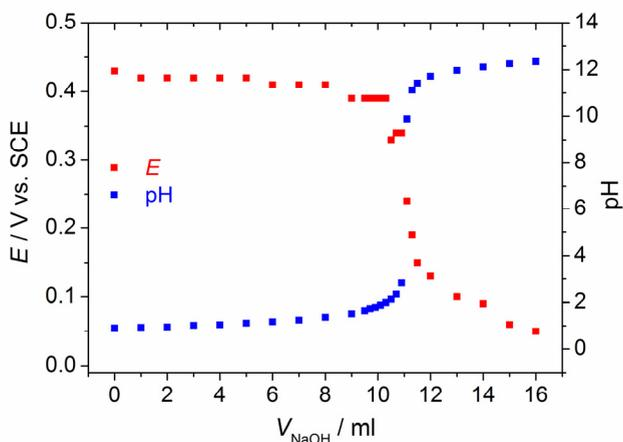
**Figure 1.** Potentiometric titration curves obtained for the titration of  $100 \text{ cm}^3$  of  $0.1 \text{ mol dm}^{-3} \text{ HClO}_4$  with  $1 \text{ mol dm}^{-3} \text{ NaOH}$  at a PIGE ( $E$  vs.  $V$  curve) and at a glass electrode (pH vs.  $V$  curve), respectively.
