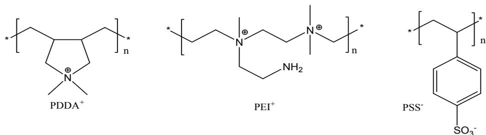
**Figure 1.** Chemical structures of commonly used charged polymers in LbL: poly(dimethyldiallyammonium chloride) (PDDA<sup>+</sup>), polyethyimine (PEI<sup>+</sup>) and polystyrene sulfonate (PSS<sup>-</sup>).
