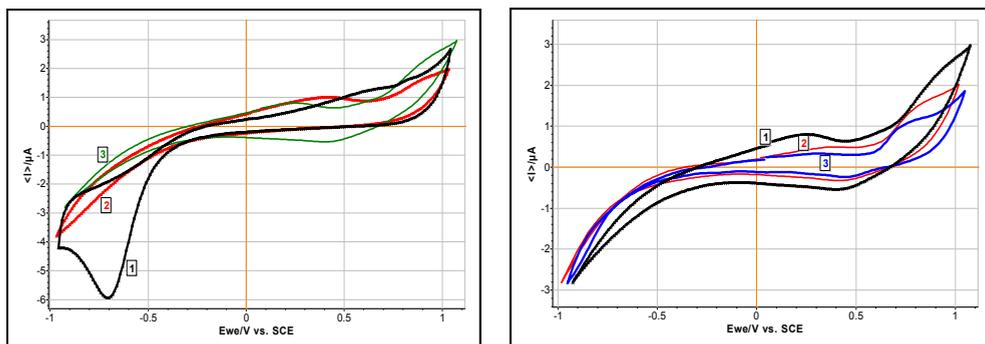
**Figure 3 (a).** Cyclic voltammograms measured in aq. Lr ranging pH: 9.0 (1); 7.0 (2) and 6.0 (3);  $E = 1 \text{ V}$ , scan rate  $100 \text{ mVs}^{-1}$ . **(b)** Cyclic voltammograms measured in aq. fresh Lr (pH 6.0) at different scan rate:  $100 \text{ mVs}^{-1}$ (1);  $50 \text{ mVs}^{-1}$ (2) and  $20 \text{ mVs}^{-1}$ (3),  $E = 1 \text{ V}$ .
