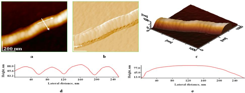
**Figure 2.** Collagen fiber transferred on glass substrate from the air/aqueous phase of 2M NaCl, at 30 mN/m. 2D topography (a), amplitude (b), 3D-topography (c), cross section profiles along the arrows in image (a), parallel with long axis of COL fiber (d) and perpendicular on COLL fiber (e). Scanned area  $1 \mu\text{m} \times 1 \mu\text{m}$ . Surface roughness (RMS) 32.3 nm, on scanned area (a).
