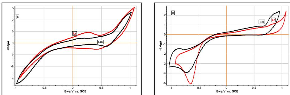
**Figure 2.** Cyclic voltammograms in aq. Lr and Lm from fresh solutions with initial pH (a) and at pH 9.0 (b);  $E = \pm 1.0$  V vs. SCE, from a negative direction, scan rate  $100 \text{ mVs}^{-1}$ (a), scan rate  $50 \text{ mVs}^{-1}$ (b).
