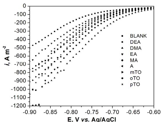
**Figure 1.** Linear voltammograms recorded on copper electrode in 0.5 M H<sub>2</sub>SO<sub>4</sub> solution at 298 K; concentration of amines: 10<sup>-3</sup> M, scan rate: 10 mVs<sup>-1</sup>.
