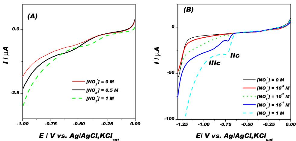
**Figure 4.** Linear scan voltammograms at G (A) and G/polyHm (B) modified electrode for different concentrations of  $\text{NO}_2^-$ . Experimental conditions: electrolyte, 0.05 M phosphate buffer + 0.1 M KBr, pH 8; scan rate,  $0.02 \text{ V s}^{-1}$ ; starting potential, 0 V vs. Ag/AgCl,  $\text{KCl}_{\text{sat}}$ ; deaerated solution (with  $\text{N}_2$ ).
