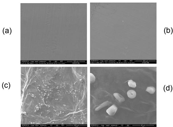
**Figure 2.** SEM micrographs of silane films deposited on aluminium substrate: (a) OTES 5%, (b) VTES 5%, (c) VTES 5% modified with CeO<sub>2</sub> and (d) VTES 5% modified with SiC
