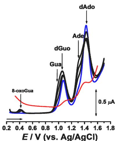
**Figure 4.** DP voltammograms in pH = 4.5 0.1 M acetate buffer with a thick multi-layer dsDNA-BDDE biosensor: (—) control and (—) first scan and (—) subsequent scans after applying + 3.0 V during 2 h to the BDDE surface causing electrogeneration of hydroxyl radicals. From reference [11] with permission.
