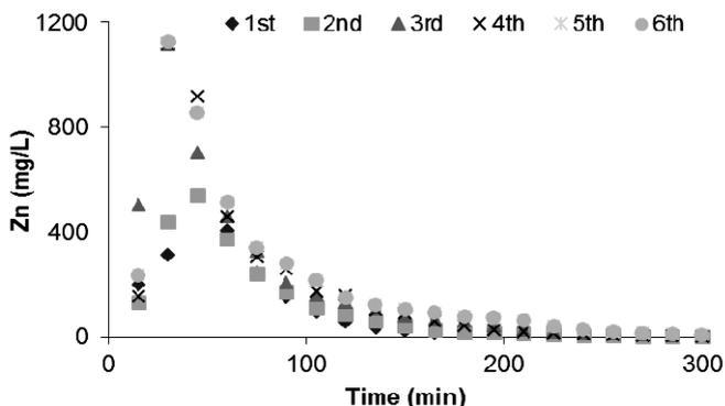
**Figure 2.** Zinc concentration during regeneration cycles in fixed bed column
