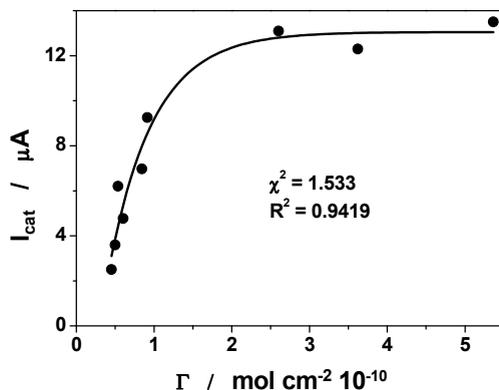
**Figure 6.** Dependence of NADH electrooxidation current on surface coverage of MB-CA/GCEs. Experimental conditions: scan rate, 2 mV/s; electrode rotation speed, 300 rpm; supporting electrolyte, 0.1 M Tris buffer (pH 7).
