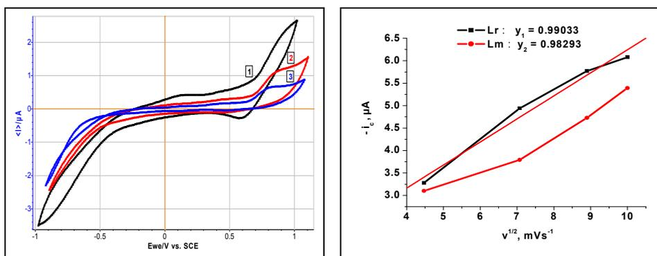
**Figure 4 (a).** Cyclic voltammograms in aq. fresh Lm (pH 5.50), at different scan rate: 100 mVs<sup>-1</sup> (1); 50 mVs<sup>-1</sup> (2) and 20 mVs<sup>-1</sup> (3), E = 1 V. **(b).** Plot of cathodic current vs. square root of scan rates.
