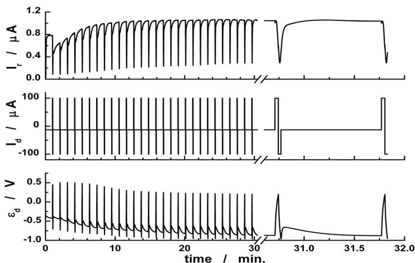
**Figure 1.** The influence of the disk applied current ( $I_d$ ) on the recorded disc potential ( $\varepsilon_d$ ) and ring current ( $I_r$ ) for 30 cycles of galvanostatic EA and HPE. ( $T_{AS} = 2$  s;  $I_{AS} = +100$   $\mu\text{A}$ ;  $T_{PRS} = 1.5$  s;  $I_{PRS} = -100$   $\mu\text{A}$ ;  $T_{PS} = 60$  s;  $I_{PS} = -13$   $\mu\text{A}$ )
