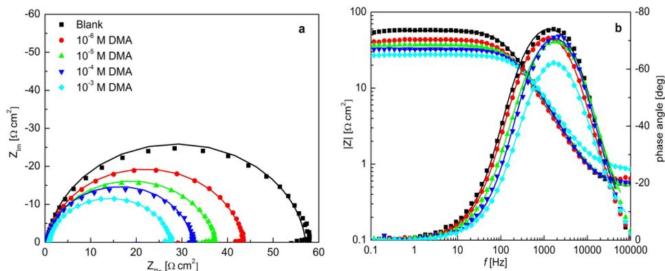
**Figure 4.** Experimental Nyquist (a) and Bode (b) plots at overpotential of -0.4 V and T = 308 K for HER on copper in 0.5 M H<sub>2</sub>SO<sub>4</sub> with different concentrations of DMA. Symbols are experimental points and continuous line are simulated by the CNLS fitting according to the electrical equivalent circuit.
