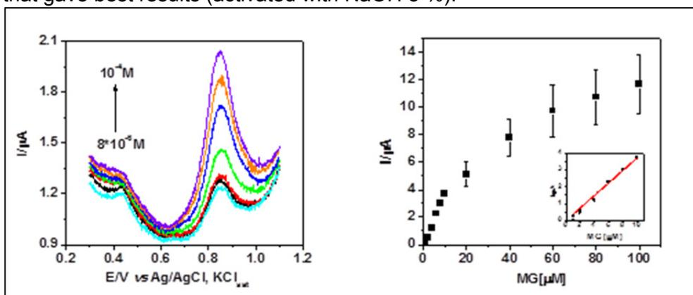
**Figure 2.** SWASV and calibration curves for **GC/AC/Nafion** electrodes prepared with AC activated with NaOH 5 %. Experimental conditions: PB 0.1M, pH 3;  $10^{-6}$  –  $10^{-4}$  M MG; frequency, 25 Hz; amplitude, 0.01 V; deposition time, 300s; start potential, 0.3 V vs. Ag/AgCl, KCl<sub>sat</sub>.
